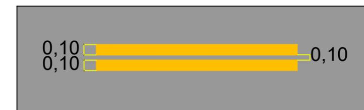
DETALHE DA PINTURA CONTÍNUA DO EIXO DA PISTA (LFO-3)
